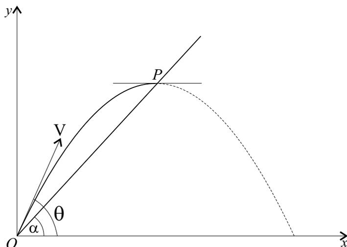
In the diagram above the point  $O$  is the foot of a plane inclined at an angle  $\alpha$  to the horizontal. A particle is projected with speed  $V$  from  $O$  at an angle of elevation  $\theta$  to the horizontal, where  $\theta > \alpha$ . It strikes the inclined plane at  $P$ , which is the vertex of the parabolic path of the particle. You may assume that this parabolic path has parametric equations  $x = Vt \cos \theta$  and  $y = Vt \sin \theta - \frac{1}{2}gt^2$ .
